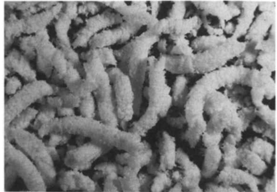
Fig. 5. Extrudate consisting of 50% \beta -lactose, 25% microcrystalline cellulose and 25% water prepared by a twin screw extruder.
