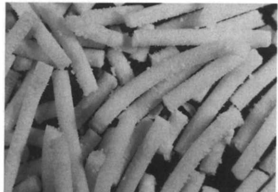
Fig. 6. Extrudate consisting of 50% \beta -lactose, 25% microcrystalline cellulose and 25% water prepared by a gravity feed extruder.
