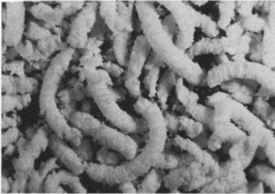
Fig. 3. Extrudate consisting of 40% \alpha -lactose monohydrate, 30% microcrystalline cellulose and 30% water prepared by a twin screw extruder.
