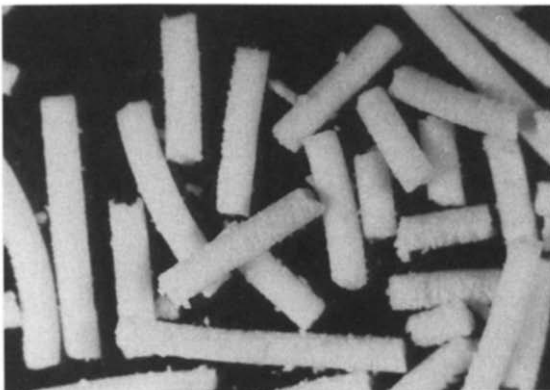
Fig. 4. Extrudate consisting of 40% \alpha -lactose monohydrate, 30% microcrystalline cellulose and 30% water prepared by a gravity feed extruder.
